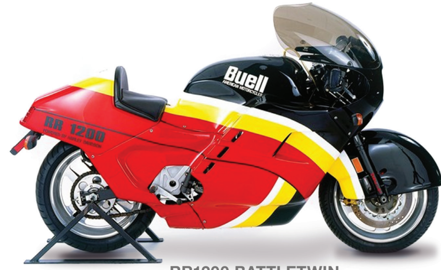
88 RR1200 BATTLEWIN MODEL YEARS PRODUCED | 1988-1990 APPROX. NUMBER BUILT | 59 HORSEPOWER@RPM | 68@6000 TORQUE (FT-LBS)@RPM | 72@4000 DISPLACEMENT | 1203
