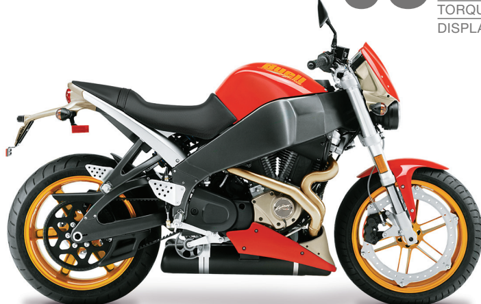
04 LIGHTNING ® XB12S MODEL YEARS PRODUCED | 2004-2008 APPROX. NUMBER BUILT | 10,852 HORSEPOWER@RPM | 103@6800 TORQUE (FT-LBS)@RPM | 84@6000 DISPLACEMENT | 1203
