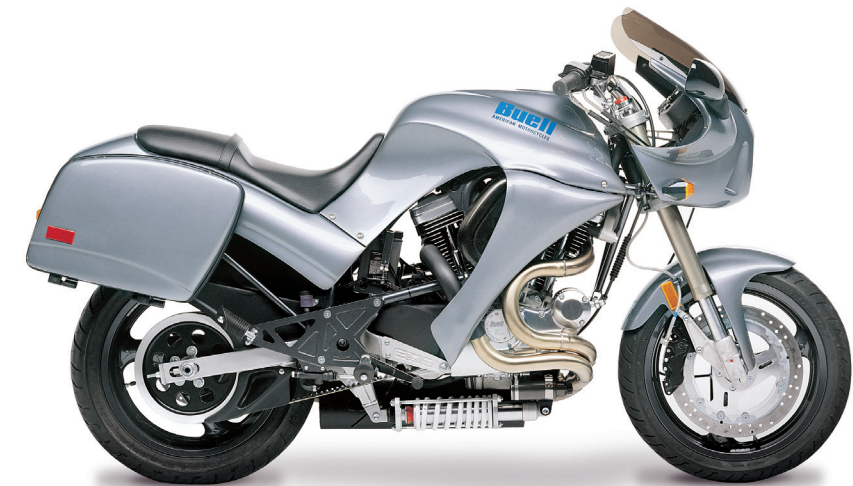
96 S2T THUNDERBOLT ® MODEL YEARS PRODUCED | 1996 APPROX. NUMBER BUILT | 429 HORSEPOWER@RPM | 76@5250 TORQUE (FT-LBS)@RPM | 78@4500 DISPLACEMENT | 1203
