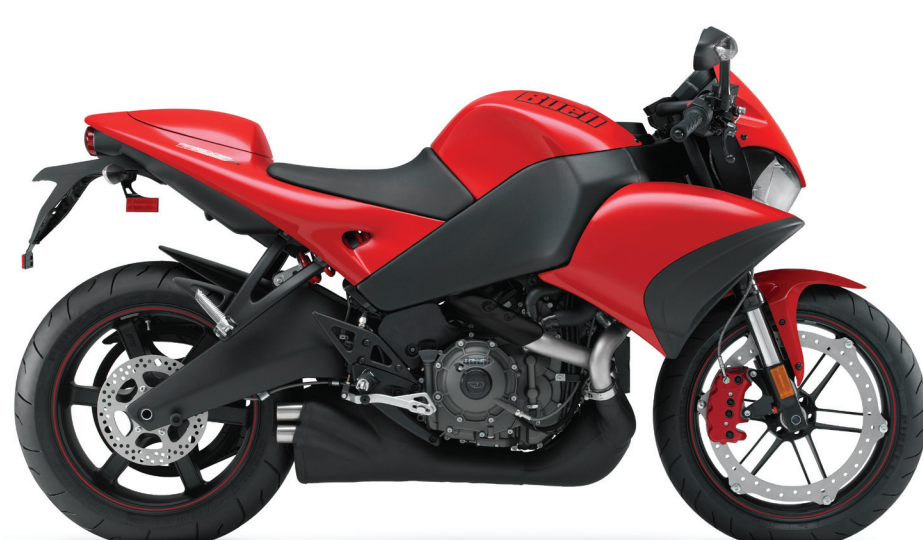
09 1125CR ™ MODEL YEARS PRODUCED | 2009-2010 APPROX. NUMBER BUILT | 3,099 HORSEPOWER@RPM | 146@9800 TORQUE (FT-LBS)@RPM | 82@6000 DISPLACEMENT | 1125
