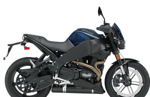
10 LIGHTNING ® CITY X XB12SX MODEL YEARS PRODUCED | 2010 (EU ONLY) APPROX. NUMBER BUILT | 860 HORSEPOWER@RPM | 103@6800 TORQUE (FT-LBS)@RPM | 84@6000 DISPLACEMENT | 1203
