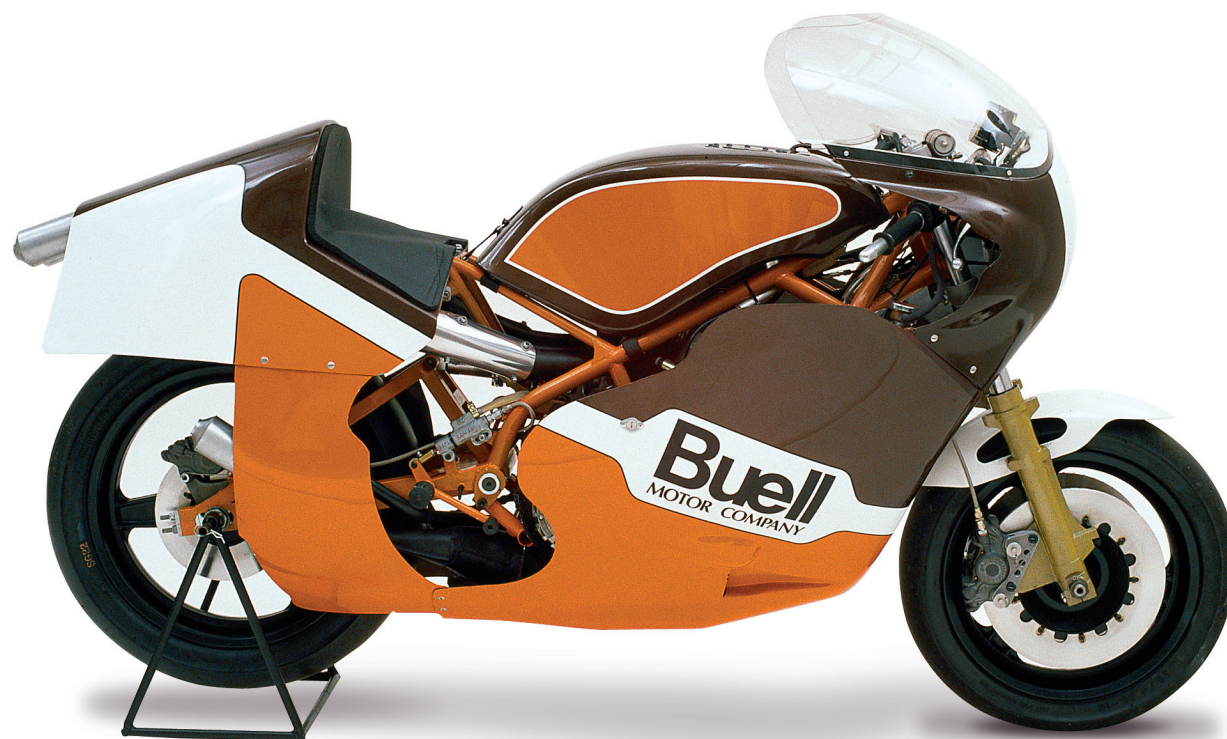
83 RW750 MODEL YEARS PRODUCED | 1983 APPROX. NUMBER BUILT | 2 HORSEPOWER@RPM | 163.5@10500 TORQUE (FT-LBS)@RPM | 83.6@9500 DISPLACEMENT | 748
