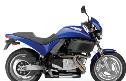
01 M2L CYCLONE ® MODEL YEARS PRODUCED | 2001-2002 APPROX. NUMBER BUILT | 1,761 HORSEPOWER@RPM | 91@6000 TORQUE (FT-LBS)@RPM | 85@4900 DISPLACEMENT | 1203
