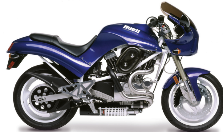
95 S2 THUNDERBOLT ® MODEL YEARS PRODUCED | 1995-1996 APPROX. NUMBER BUILT | 1,694 HORSEPOWER@RPM | 76@5250 TORQUE (FT-LBS)@RPM | 78@4500 DISPLACEMENT | 1203
