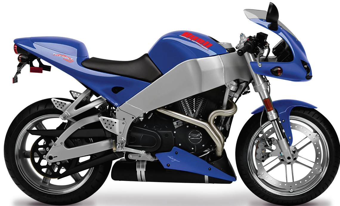
03 FIREBOLT ® XB9R MODEL YEARS PRODUCED | 2003-2007 APPROX. NUMBER BUILT | 7,461 HORSEPOWER@RPM | 92@7500 TORQUE (FT-LBS)@RPM | 68@5500 DISPLACEMENT | 984
