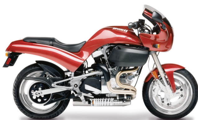
97 S3 THUNDERBOLT ® MODEL YEARS PRODUCED | 1997-2001 APPROX. NUMBER BUILT | 2,672 HORSEPOWER@RPM | 91@5800 TORQUE (FT-LBS)@RPM | 87@5200 DISPLACEMENT | 1203
