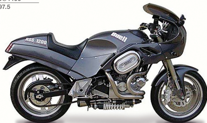
91 RSS1200 WESTWIND MODEL YEARS PRODUCED | 1991-1992 APPROX. NUMBER BUILT | 38 HORSEPOWER@RPM | 68@6000 TORQUE (FT-LBS)@RPM | 72@4000 DISPLACEMENT | 1203
