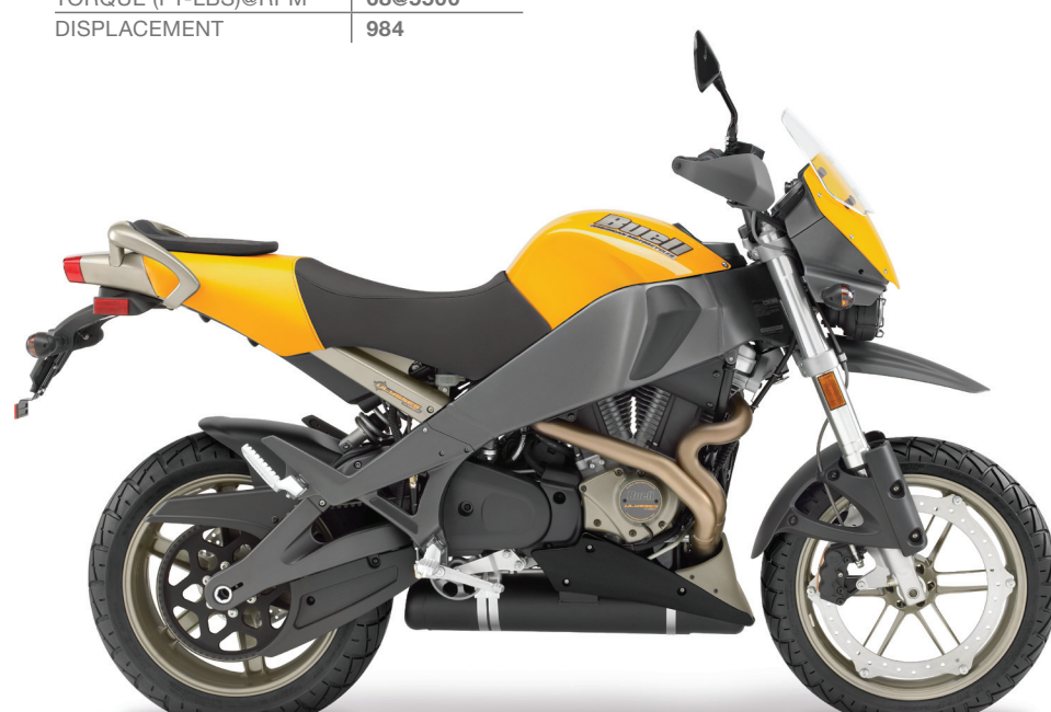
06 ULYSSES ® XB12X MODEL YEARS PRODUCED | 2006-2010 APPROX. NUMBER BUILT | 7,432 HORSEPOWER@RPM | 103@6800 TORQUE (FT-LBS)@RPM | 84@6000 DISPLACEMENT | 1203
