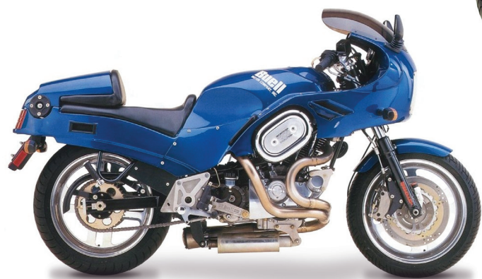
89 RS1200 WESTWIND MODEL YEARS PRODUCED | 1989-1992 APPROX. NUMBER BUILT | 208 HORSEPOWER@RPM | 68@6000 TORQUE (FT-LBS)@RPM | 72@4000 DISPLACEMENT | 1203
