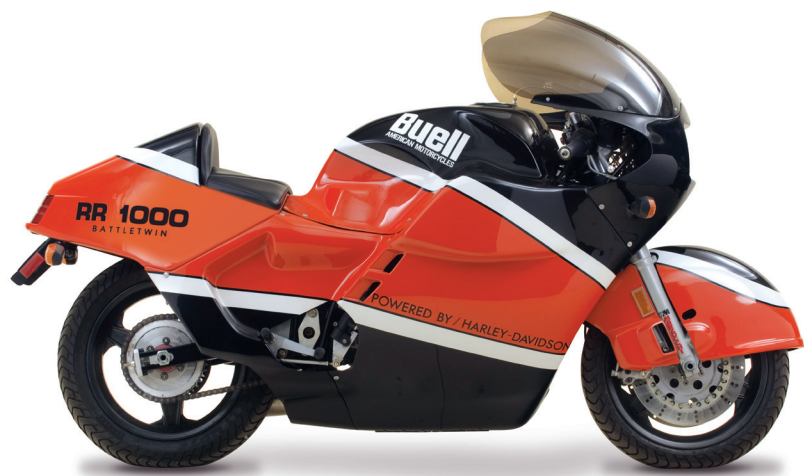
87 RR1000 BATTLEWIN MODEL YEARS PRODUCED | 1987 APPROX. NUMBER BUILT | 51 HORSEPOWER@RPM | 70@5600 TORQUE (FT-LBS)@RPM | 70@4400 DISPLACEMENT | 997.5
