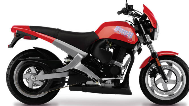
00 BLAST ® MODEL YEARS PRODUCED | 2000-2010 APPROX. NUMBER BUILT | 22,785 HORSEPOWER@RPM | 34@6500 TORQUE (FT-LBS)@RPM | 30@5500 DISPLACEMENT | 492
