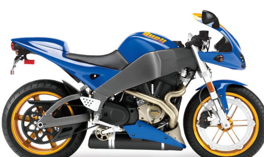
04 FIREBOLT ® XB12R MODEL YEARS PRODUCED | 2004-2010 APPROX. NUMBER BUILT | 10,408 HORSEPOWER@RPM | 103@6800 TORQUE (FT-LBS)@RPM | 84@6000 DISPLACEMENT | 1203
