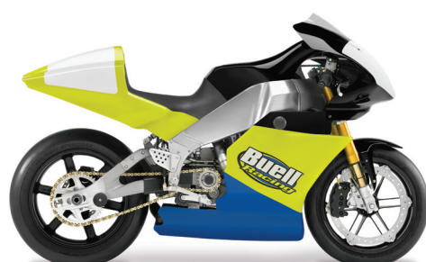
07 XBRR MODEL YEARS PRODUCED | 2007 APPROX. NUMBER BUILT | 150RW@8000 HORSEPOWER@RPM | 100@6400 DISPLACEMENT | 1338
