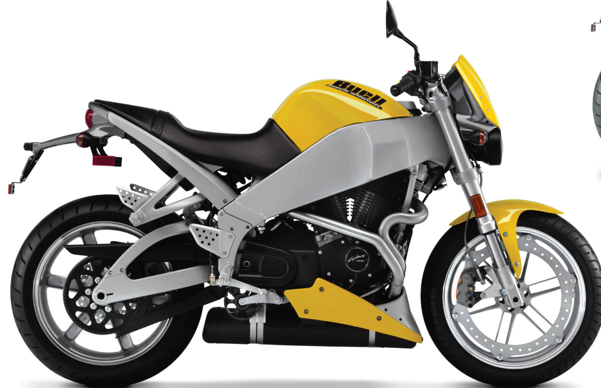
03 LIGHTNING ® XB9S MODEL YEARS PRODUCED | 2003-2004 APPROX. NUMBER BUILT | 4,332 HORSEPOWER@RPM | 92@7500 TORQUE (FT-LBS)@RPM | 68@5500 DISPLACEMENT | 984
