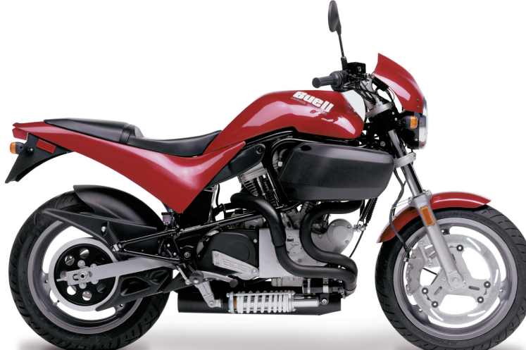
97 M2 CYCLONE ® MODEL YEARS PRODUCED | 1997-2002 APPROX. NUMBER BUILT | 8,803 HORSEPOWER@RPM | 83@5800 TORQUE (FT-LBS)@RPM | 80@4500 DISPLACEMENT | 1203
