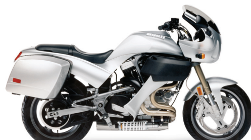
97 S3T THUNDERBOLT ® MODEL YEARS PRODUCED | 97-98, 00-02 APPROX. NUMBER BUILT | 1,779 HORSEPOWER@RPM | 91@5800 TORQUE (FT-LBS)@RPM | 87@5200 DISPLACEMENT | 1203
