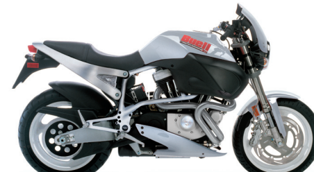
00 X1M LIGHTNING ® MILLENNIUM MODEL YEARS PRODUCED | 2000 APPROX. NUMBER BUILT | 661 HORSEPOWER@RPM | 101@6000 TORQUE (FT-LBS)@RPM | 90@5500 DISPLACEMENT | 1203
