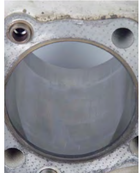
No mercy: Wear marks in the coating of the cylinders, perhaps caused by careless warming-up
